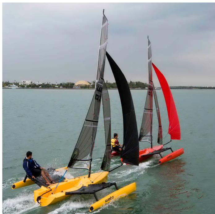
The boat is lightweight, quick and easy to rig and packs up to the size of a laser for transport and storage. Fully rigged it only weighs 220 lbs (100 kg) and can be ready to sail in less than 20 minutes. There are only five lines to control all three sails and the mast is so light that kids can rig the Weta and launch it effortlessly from the specially-designed trailer.
