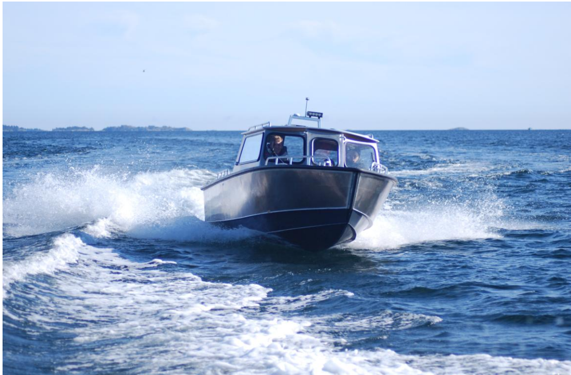
Boat dual chines and a narrow planing bottom with low deadrise
