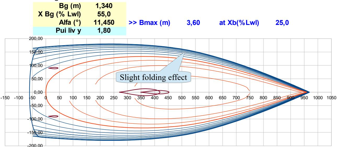
That folding effect, created when Pui liv y < 2, is well showed by the curvature 1/R curve also given in the output, the sheer line 1/R being the thick blue line here below :
