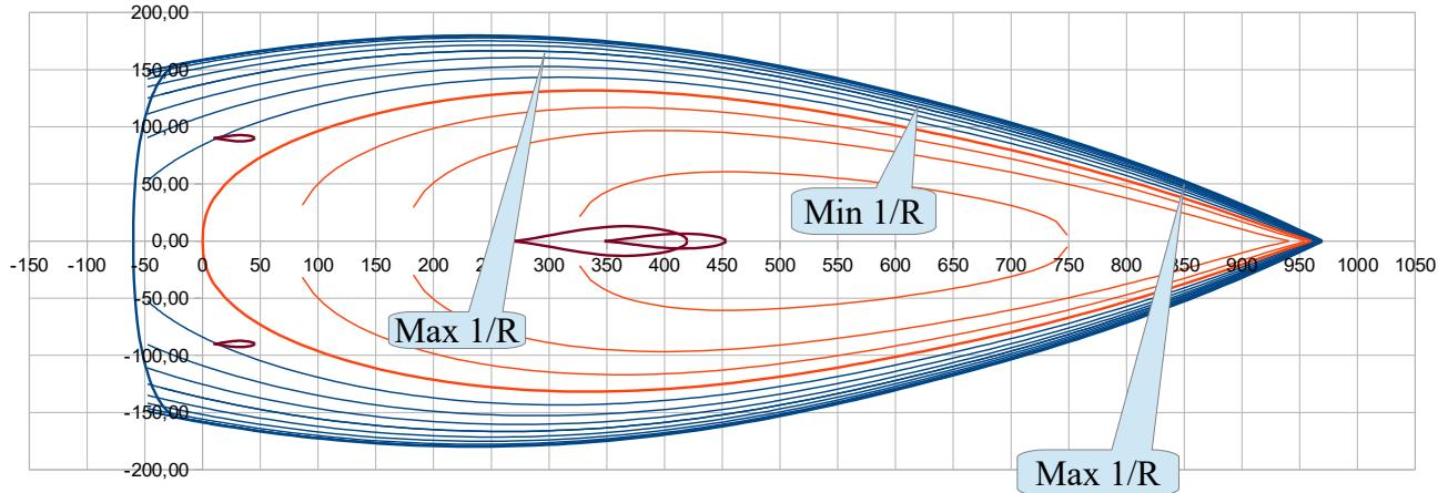
Here the existence of the 2 maxima of curvature is more visible on the sheer line and well showed by the 1/R curve (the blue thick line) :
