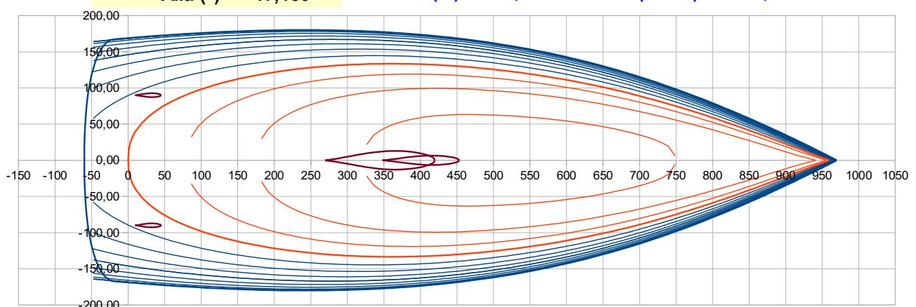
One can see that the maximum curvature of the sheer line moves forward with X Bg. At this stage, one can consider that an X Bg between 60 and 70 can give a good shape, so let's consider **X Bg = 65** :
