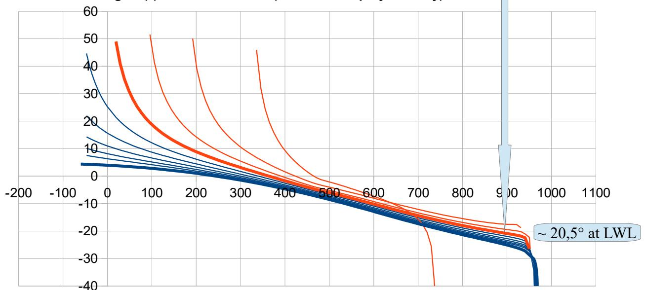
>>> One can evaluate the entry half-angle at the X position where the curvature is minimum before increasing sharply at very fore end due to the roudness : this angle is  $\sim 20,5^{\circ}$  for the LWL, which is within the usual ones for cruising yachts.
