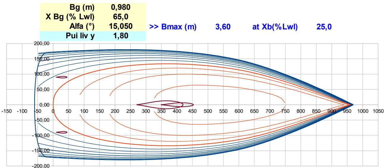
Here, the folding effect is moderated and could be more relevant if we can put it a bit aft, so this variant with X Bg = 55 :
