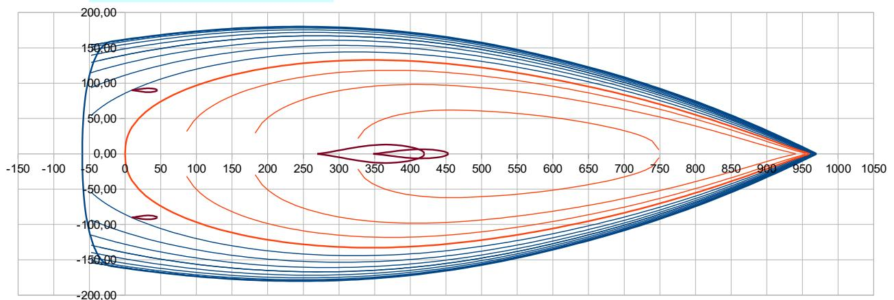
When Pui liv y > 2 , that creates 2 maxima of the curvature along the sheer line, it is imperceptible on the drawing but well showed by the curvature 1/R curve :
