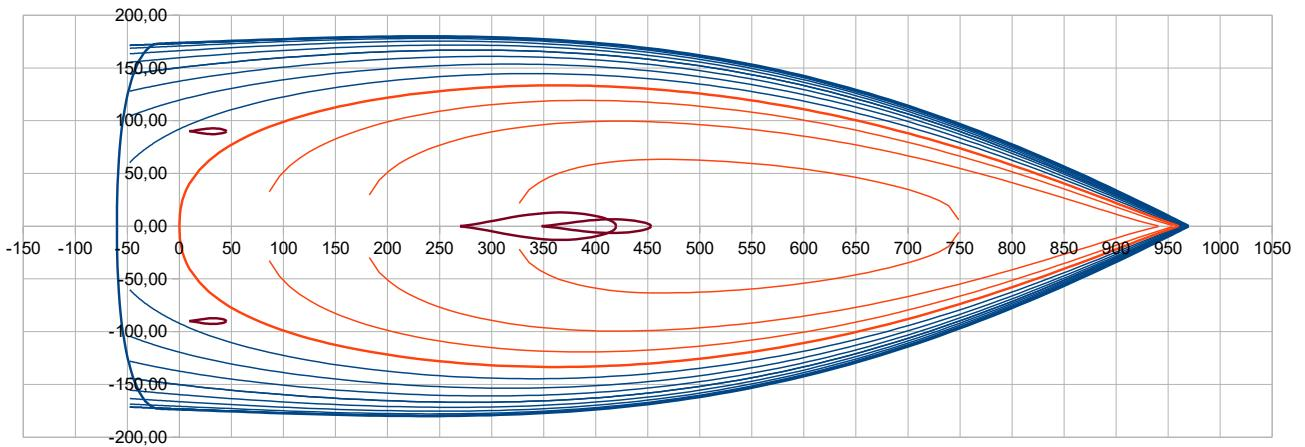
One can see from the curvature  $1/R$  curve that the rear end of the sheer line is flat (even with a slight inflection point) :
