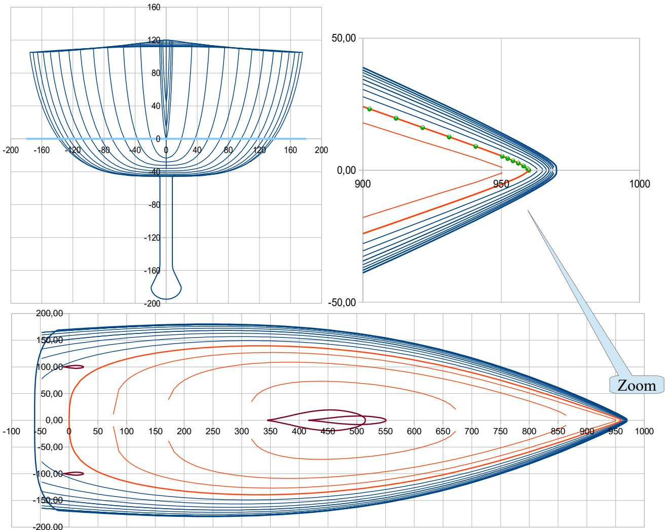
The bow waterlines, LWL and above, are not pinched before the transition to the very end roundness. Only the first waterline below the LWL shows a slight pinched, but it is ok.
