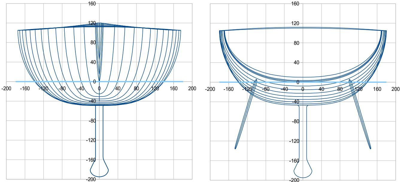
**\*15\* Keel line aft part adjustment, using the height of the rear end of the transom Z tab ar**
