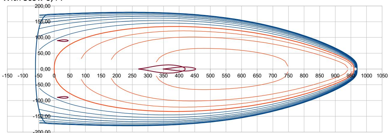
At this stage, one can consider that with « Scow » = 0,06 we have the requested small roundness at the bow very end, representative of the real building of the hull. Summarize of the sheer line data finally adopted and a first evaluation of the entry half-angle of the waterline (angles are also given in the output) :
