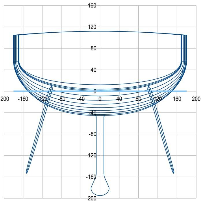
>>> one can note that the hard chine, i.e. the transition between the vertical and the round shapes of the sections, is actually very soft although it affects the whole volume and characteristics.
