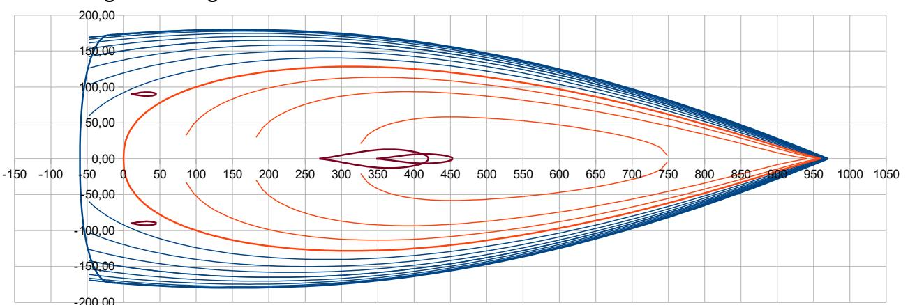
At this point, one can consider that the Bmax is a bit too aft, at 16% Lwl instead of about 25 %, so one can increase Bg and decrease alfa up to reach this objective :
