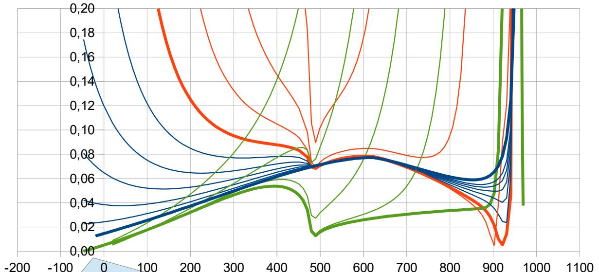
$1/R = 0$  at the end >>> no curvature at the end of the keel and buttock lines
