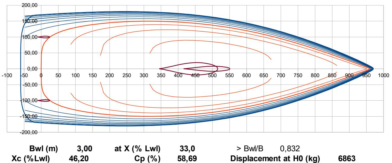
Ratios evolves towards the objectives, but the displacement is a lot too much at 6863 kg, so the second step is to reduce the power of this U rear shape , i.e. to decrease Pui U ar. >>> with **Pui U ar = 8** and a slight reduction of the hull draft **Tc to 0,463 m**, the ratios and the displacement converge towards the objectives :
