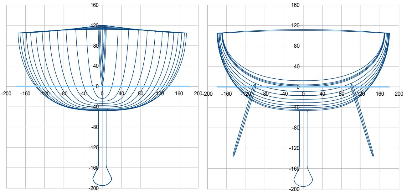
At this stage, we have the objectives to move more aft the LCB (< 47 % Lwl at least, according to PYD recommendation to minimise the residuary drag), while maintaining Cp around 0,58-0,59 (to favor high speed of planning if any), and a ratio Bwl/B that could be at least 0,77 (for the righting moment).
