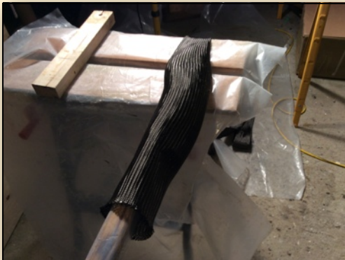
A layer of carbon braid is "pushed" on, so that it expands.
