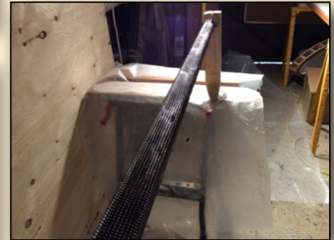
Having wetted out the outer layer with a slight excess of resin, the two layers of carbon braid are "milked" firmly, with gloved hands, from the small end towards the large end. The surface should feel uniformly wet and slippery.
