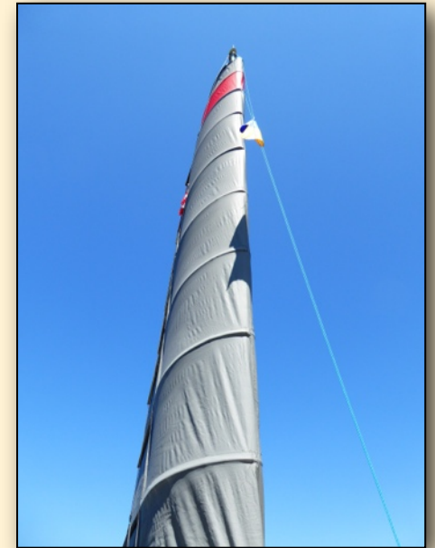
The "Holy Grail" - a sail with the efficient planform and foil section of an aircraft wing, but which has the easy handling of a junk sail.
