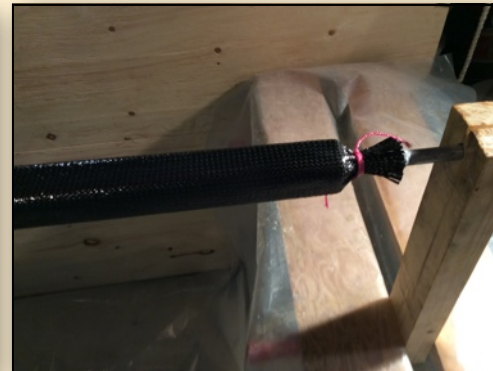
The inner layer is tied at the small end, and thoroughly wetted out.
