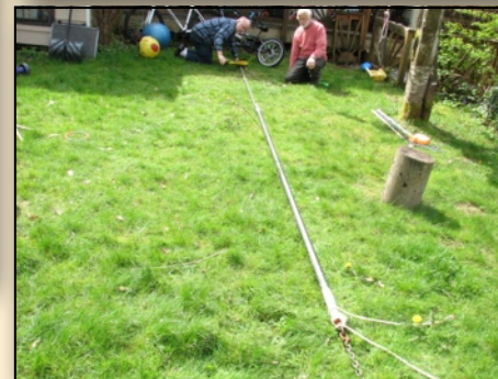
When cured, the peelply is stripped off and the mandrel is pulled out using a chain hoist, or a 4WD vehicle.
