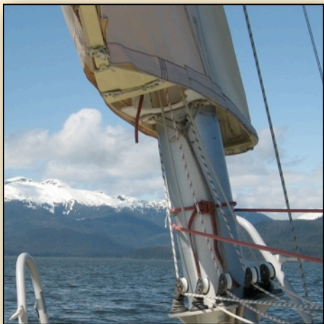
2008 - the bottom batten of the mainsail, in SE Alaska. Wishbone sides of 50 x 5mm pultruded GRP, hinge box of filament-wound GRP, luff former of moulded GRP, mast bearing of HDPE, after batten of 1 1/2" square pultruded GRP tube.
