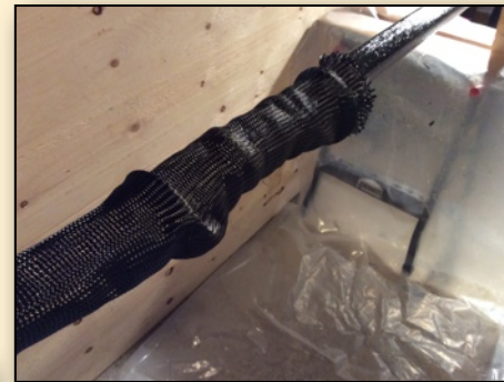
The outer layer is untied, smoothed out over the inner layer and tied at the small end. There should be an excess of resin in the inner layer, which then appears on the surface of the outer layer, indicating that the inner layer has been fully wetted out.
