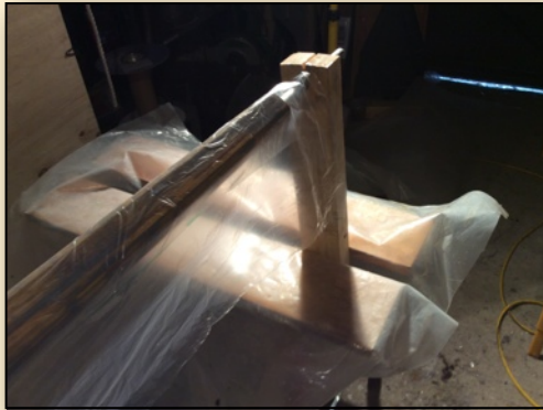
The mandrel is coated with Vaseline, and a strip of thin plastic film is wrapped around it.
