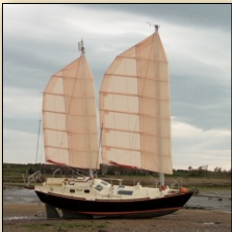
Early 2005 - the newly fitted ketch wing sail rig in Ravenglass Harbour. The mainmast in the original position, the mizzen mast added just forward of the companionway.
