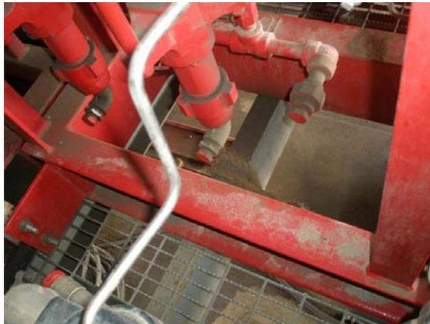
**7.7** BOP control unit air pump discharge lines not connected.
