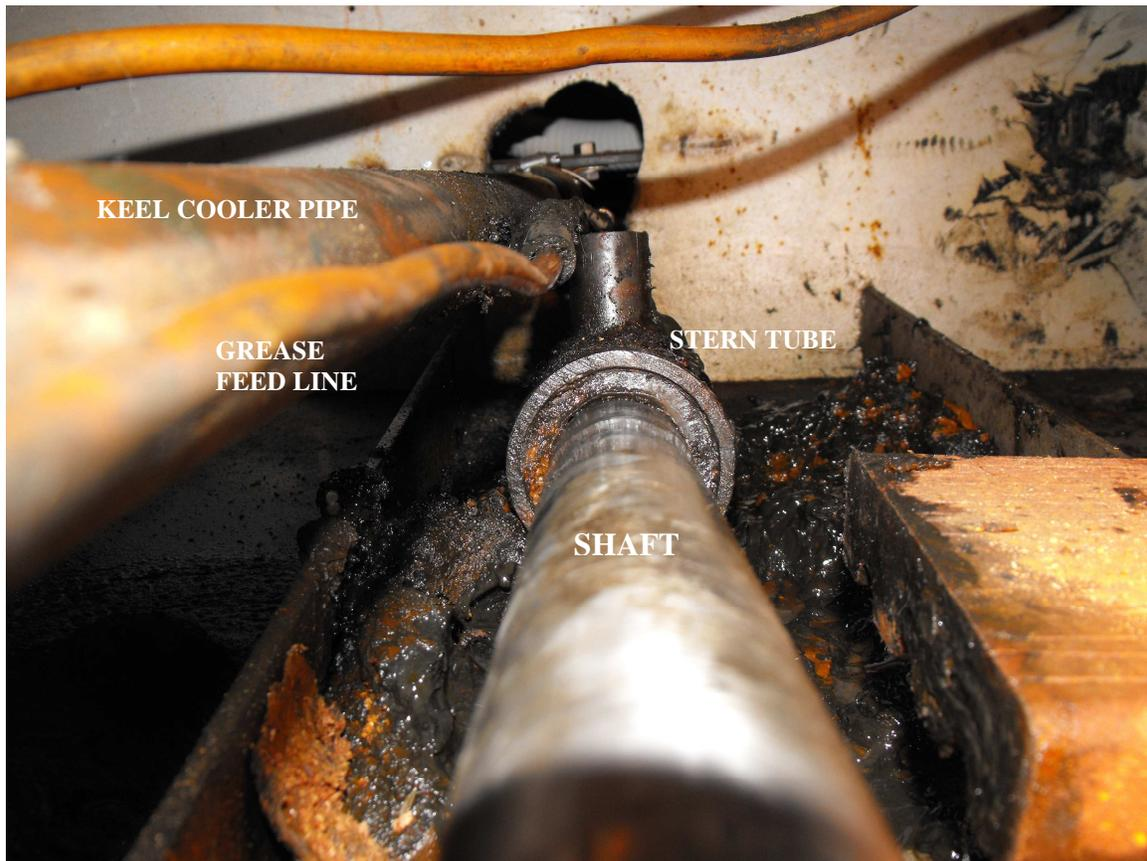
**BOTTOM OF SHAFT INTO STERN TUBE**
