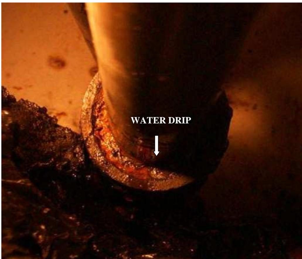
**HORIZONTAL VIEW OF SHAFT INTO STERN TUBE**
