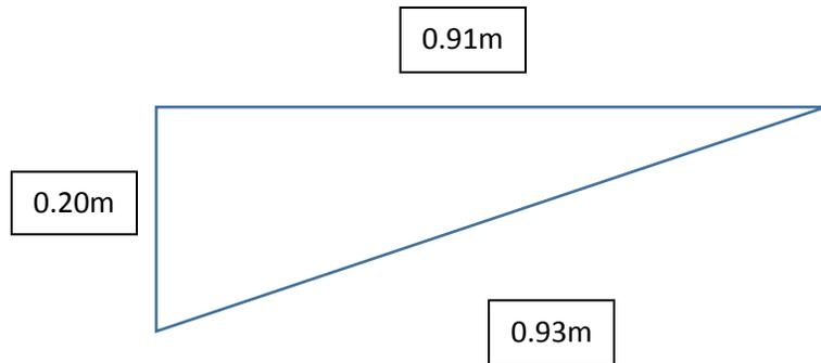
We know from the drawings above that the left hand side of the triangle is actually experiencing a force of 16000N. So we can multiply all the dimensions on the triangle by a factor to get 16000 on the left side.
