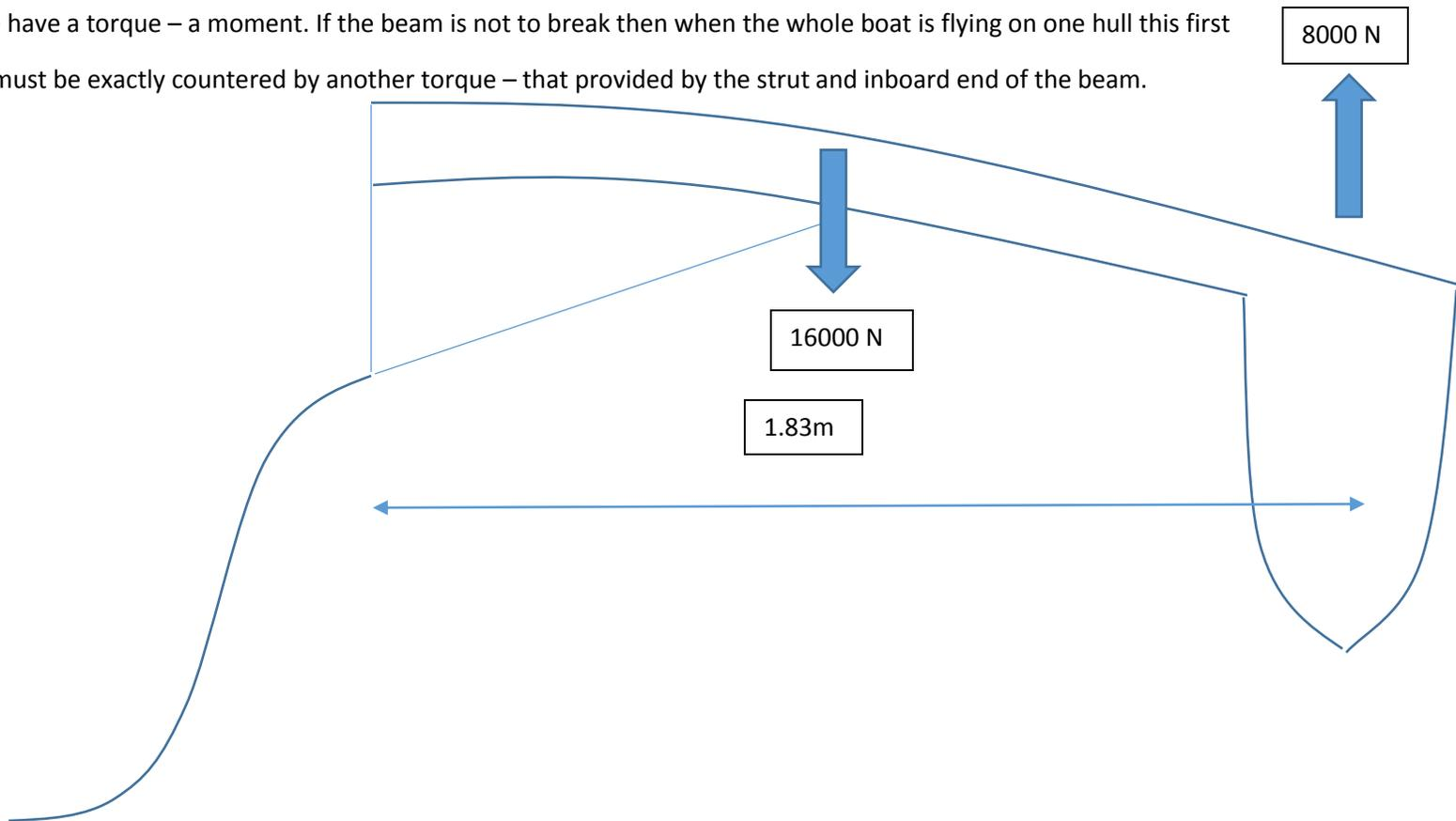
If we estimate that the strut is attached halfway along the beam we can use similar triangles to calculate the different components. First off we have to remember that the strut has to pull down vertically TWICE the weight of the boat as it is only half as far along the beam as the float. This is why my old Twiggy had its underwires attached to the end of the beam.
