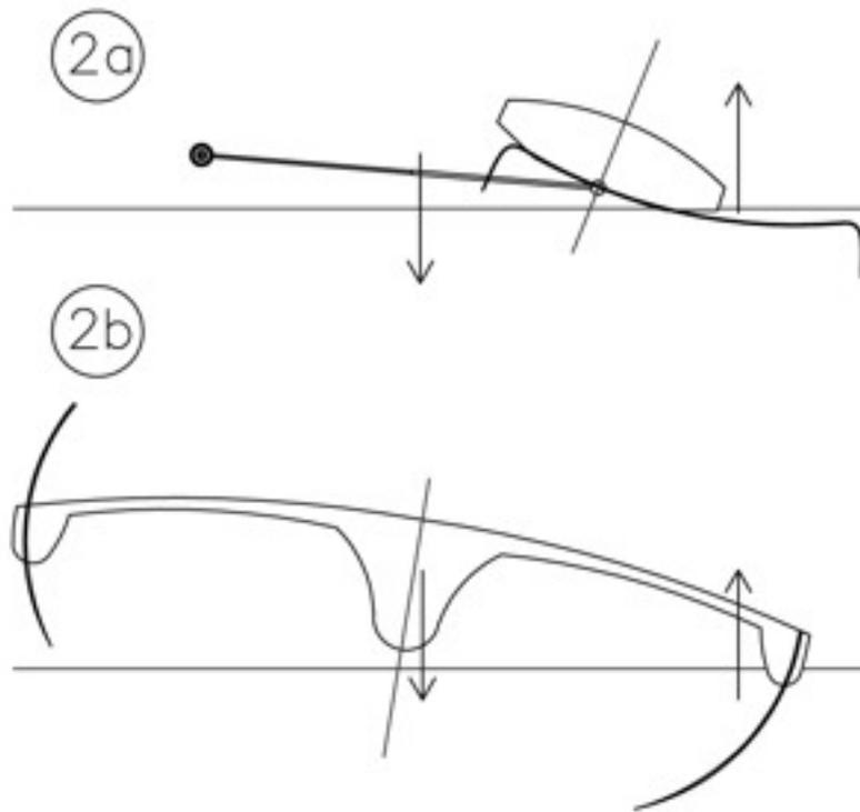
SpeedDream's foil partially lifts the boat out of water and significantly increases her stability by moving the forces of dynamic support to leeward. In a similar way the addition of a curved foil to the multihull float helps to lift the boat and reduce drag, but it also reduces stability by moving forces of dynamic support inboard. This greatly exacerbates the main problem faced by offshore multihulls; the lack of ultimate stability.
