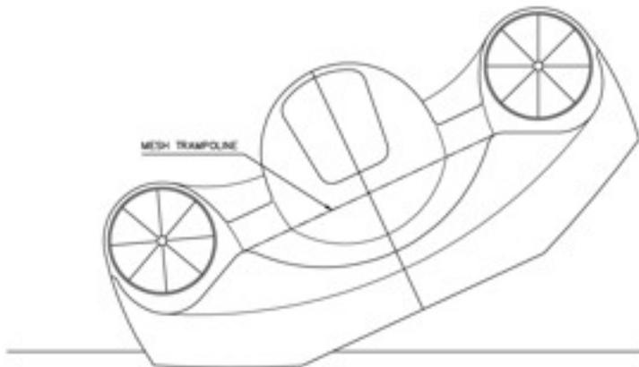
catamaran but of critical importance, when it comes to speed at least, is the relative shapes of the immersed hulls. The leeward hull of a multihull is slab sided with a rounded bottom, which because of the downward force of the rest of the boat, is
