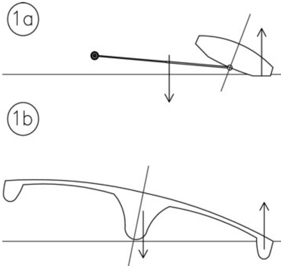
While theoretically it is possible for SpeedDream to match the righting moment of a similarly sized multihull by further extending her telescopic keel, it is really unnecessary. When sailing at high speed, a planing hull's wetted surface – and her drag – would be about half that of similarly sized multihull. Even with a smaller righting moment and smaller sail area, SpeedDream would be capable of reaching higher speeds. Her high performance is derived from efficiency rather than from power.
