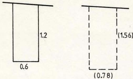
Assume existing design with  $AR_G = 2$  (Assumed  $AR_E = 4$ ) with chord 0.6 m span 1.2 m (hence area  $0.72 \text{ m}^2$ ) is required to operate at  $10^\circ$  attack in order to produce the desired sideforce at say 6 knots (3.09 m/s)
