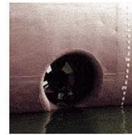
Example Radiused Tunnel Inlet
