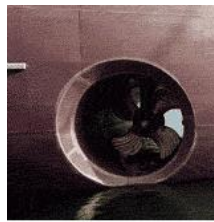
Example Chamfered Tunnel Inlet
