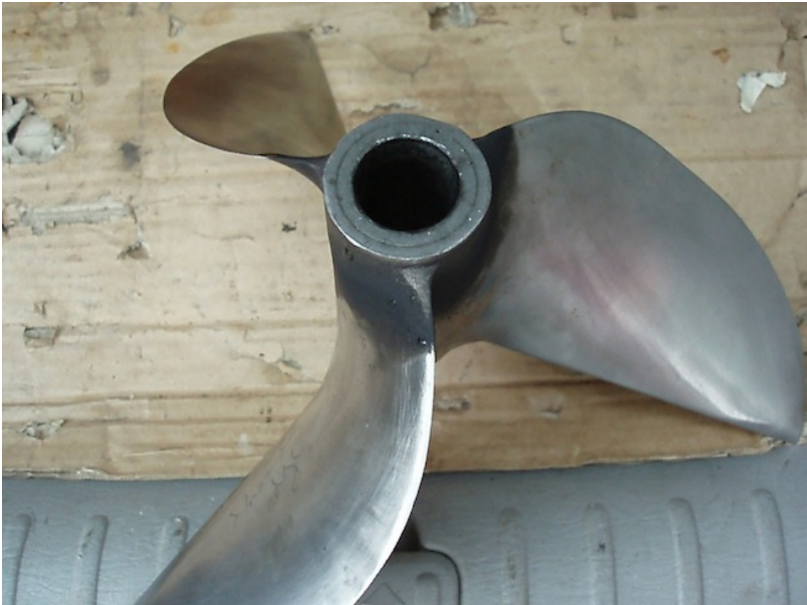
Fig. 4 EP Class prop showing no exhaust deposits where the blades were wet.
