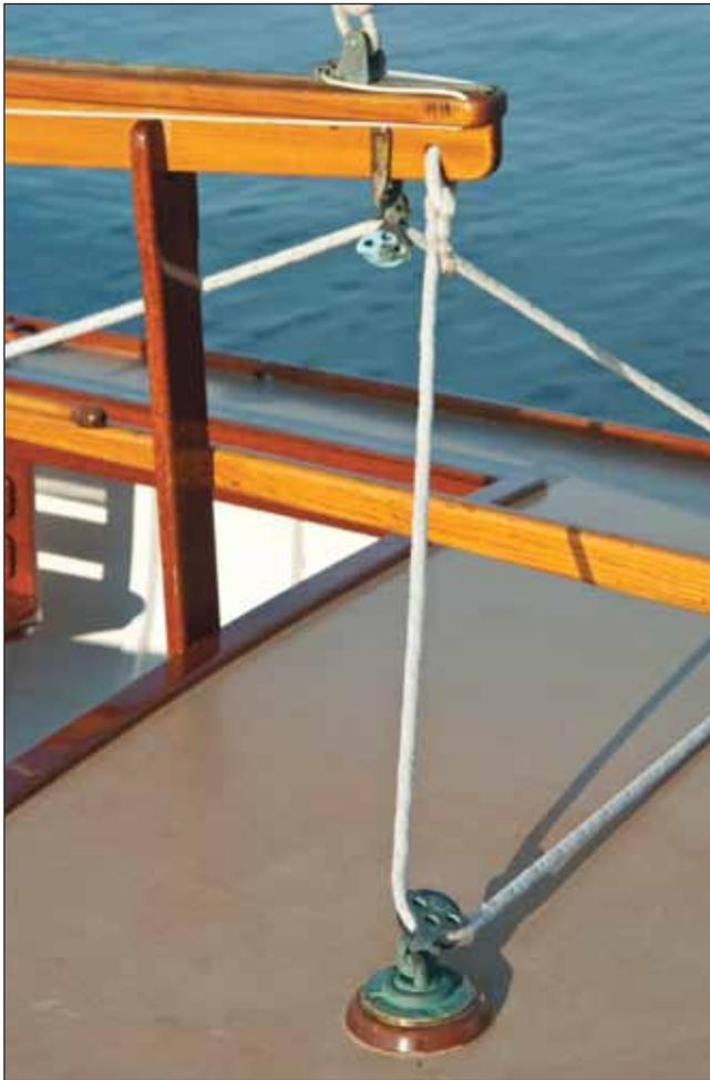
**In the original rigging plan, which is retained in SWIFT, the boom has a “T” cross-section, and the mainsheet reeves through deck-mounted turning blocks without a traveler.**
