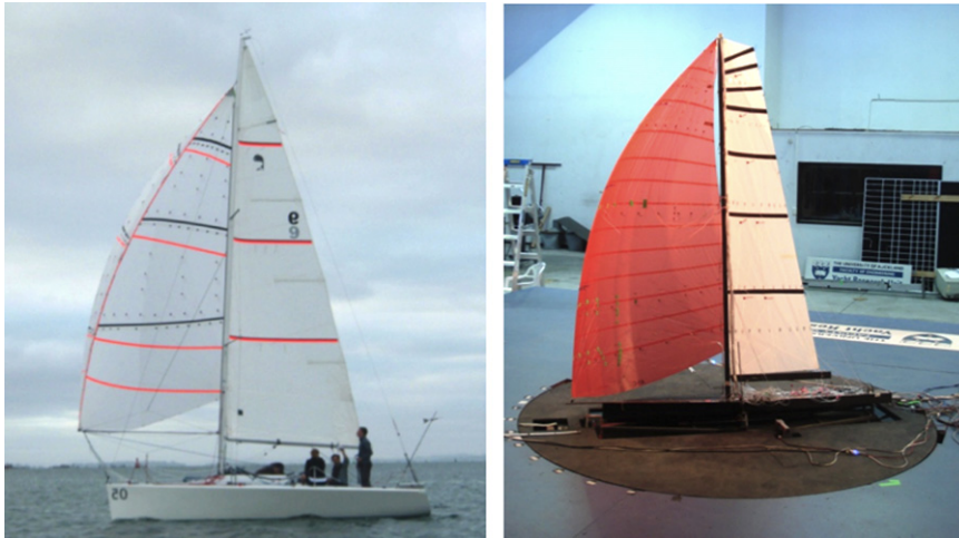
Fig. 2. Downwind sailing configurations for the pressure measurements: on-water (Platu-25 left) and wind tunnel (right). In the full-scale tests, the mainsail was reefed slightly in order to align the top of the spinnaker and mainsail to the same height.
