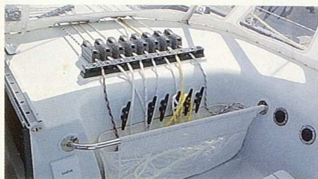
Top left , two telescopic poles are concealed by hinged bow section doors. This pole is extended to keep the anchor clear of the bow; the other is the asymmetric spinnaker pole. Above , venturi slots connected to the cockpit drains smooth the transition into higher speed ranges. Left , all rope clutches are backed up with horn cleats. Below left , the transom folds down to reveal a small RIB stowed under the after deck. Below right , the gooseneck arrangement
