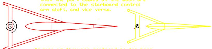
As long as they are centered on the boom... That is the clever bit with the cut outs and the roller inside the boom. Ease the roller forward and the deltas will lag behind the boom/ This reduces flap angle aloft, and simulates twist.
