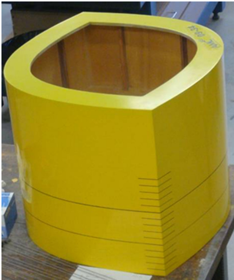
Fig. 4 Model 09-34 parabolic pressure source of 700 mm length, 600 mm beam, and 500 mm height
