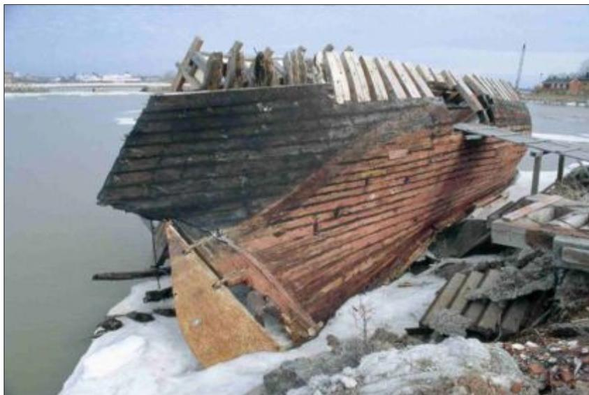
*The Alma built 1882 is the only remaining Finnish "Jakt". Until the late 1950s such ships worked as traders and were common in Finnish waters. This photo shows the condition in which she was found in 1998 on the Suomenlinna Island outside of Helsinki.*
