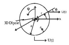
K.B.C on sphere:  $\left. \frac{\partial \phi}{\partial r} \right|_{r=a} = U(t) \cos \theta$
