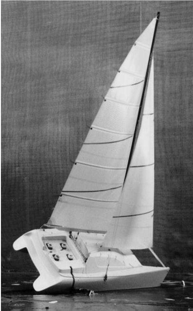
Figure 3. The model undergoing wind tunnel tests in configuration 5.
