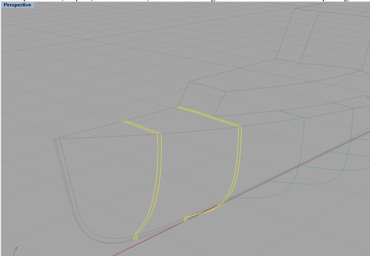
Split by sheerline and rabbet line, it's for different offset distances of the hull frame and the deck frame. It's probably vice to move the frame now to a new layer, and set only it visible. After some offsetting and trimming, it looks like this:
