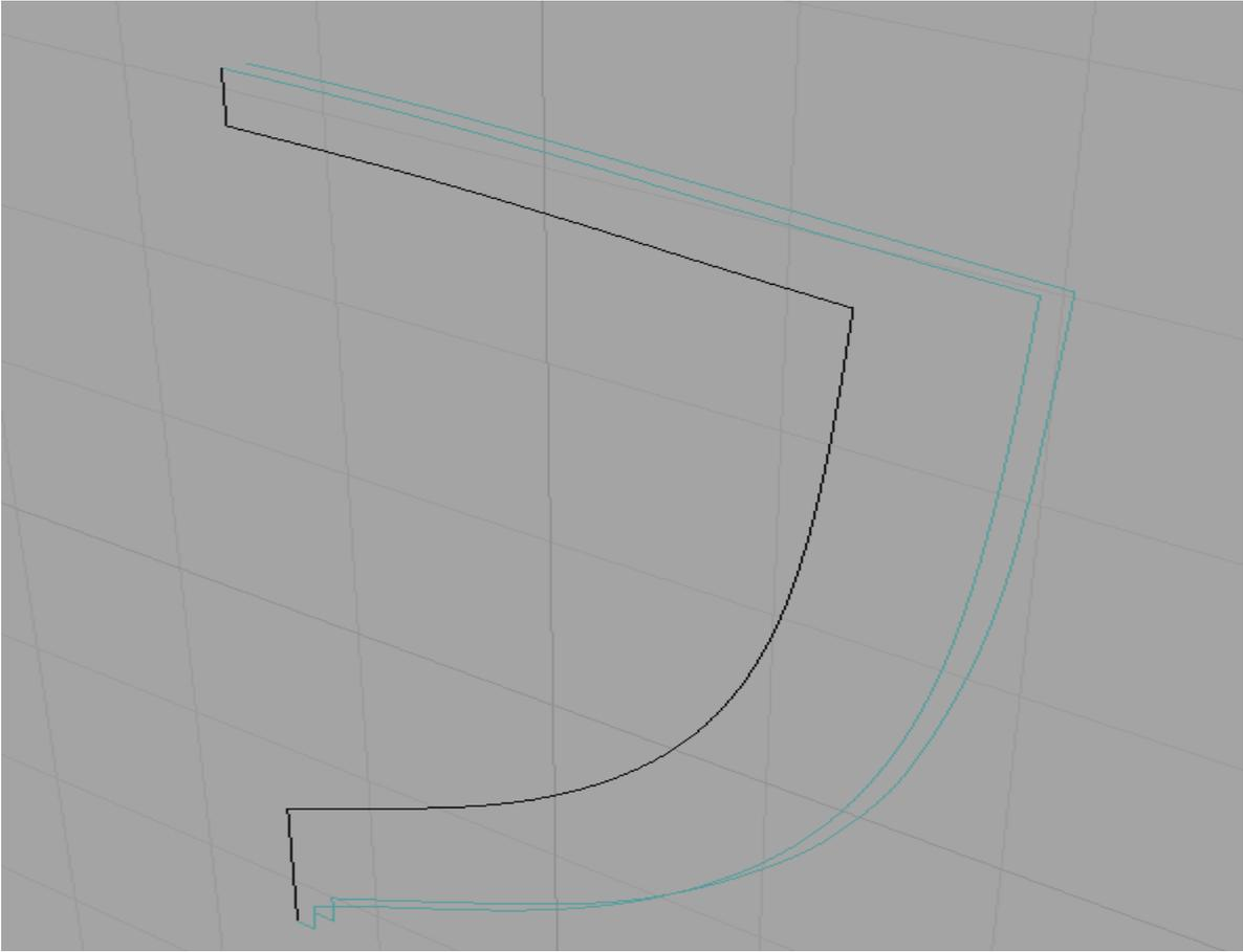
Then, extrude frames interior edges to frame thickness, here -25mm. In this way, there will be no bevel inside the frame.
