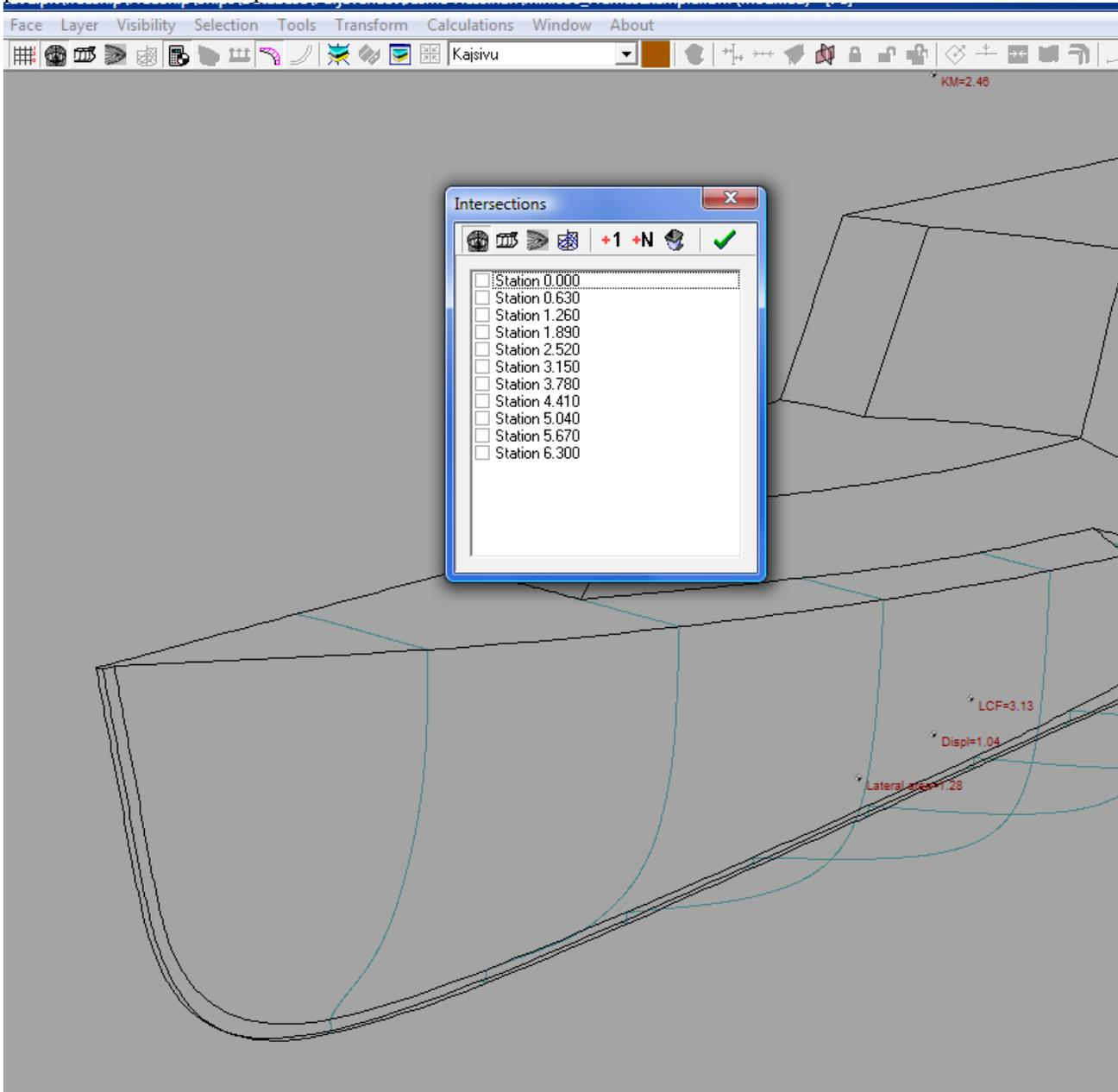
Then, the additional stations for the bow side of the frames, those being checked in the image. I used 25 mm for the frame thickness:
