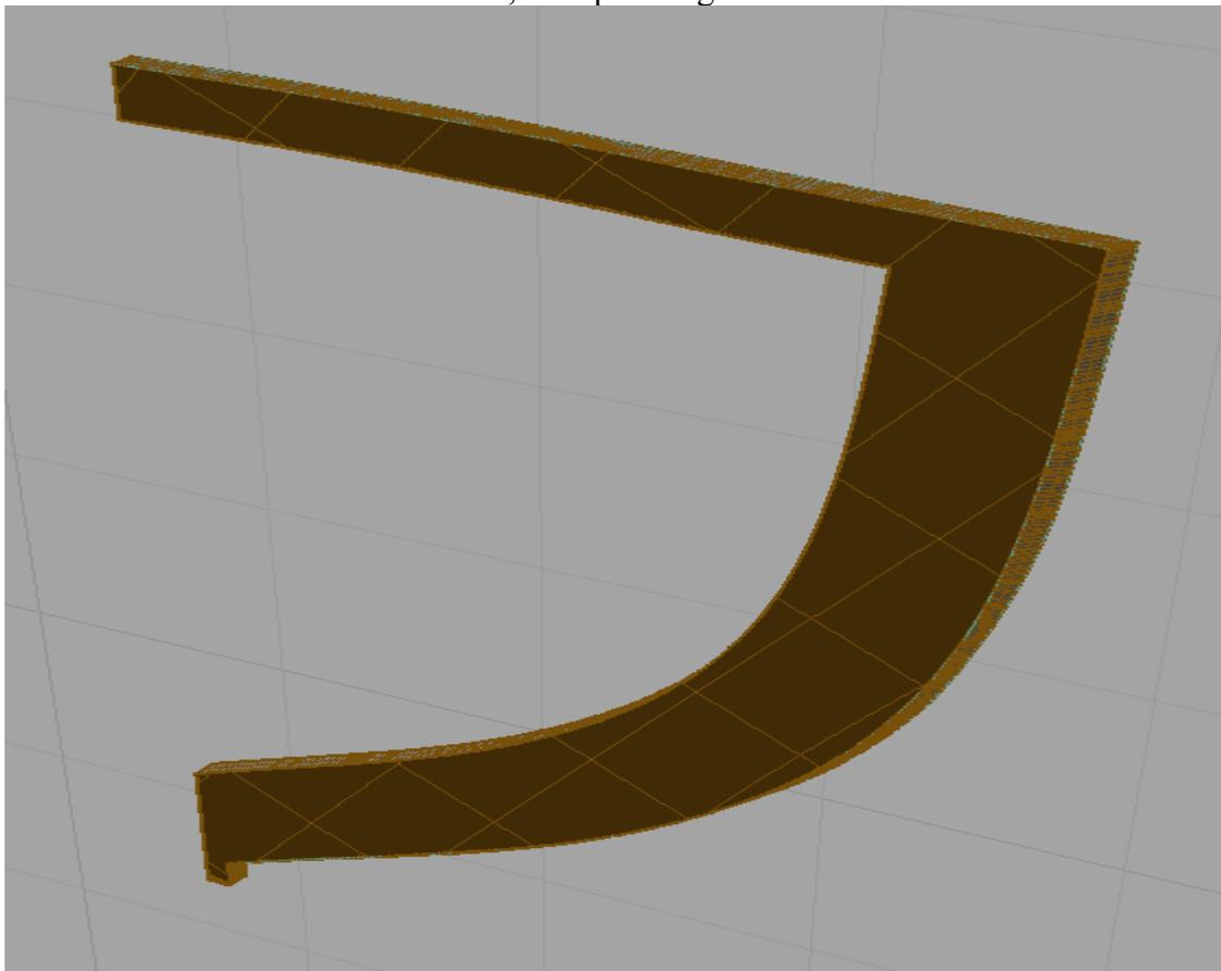
And lofted the faces against planking. Depending on your CNC-program, it isn't always necessary to make the frame solid, so I'm not creating the stern face of the frame. Now add whatever notches
