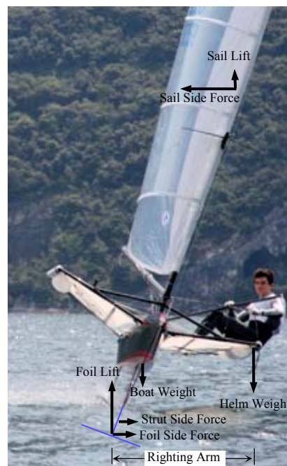
Figure 25 – Force Diagram when heeling to windward
