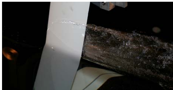
Figure 18 – Spray Generation off the Vendor2 Daggerboard T-Foil at 20 fps
