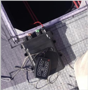
Battery Bank Good for 3-4 hours of Racing
