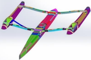
Finite Element Mesh >200 distinct ply regions for iterations which ultimately translated into construction drawings
