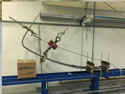
Load Testing Validation of Main Daggerboard
