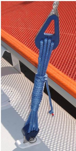
Now to clean up the lashing, just wrap the excess line around the parallel lines, continuing up the lashing. Then tuck the lashing under itself 2 or 3 times to secure it.
