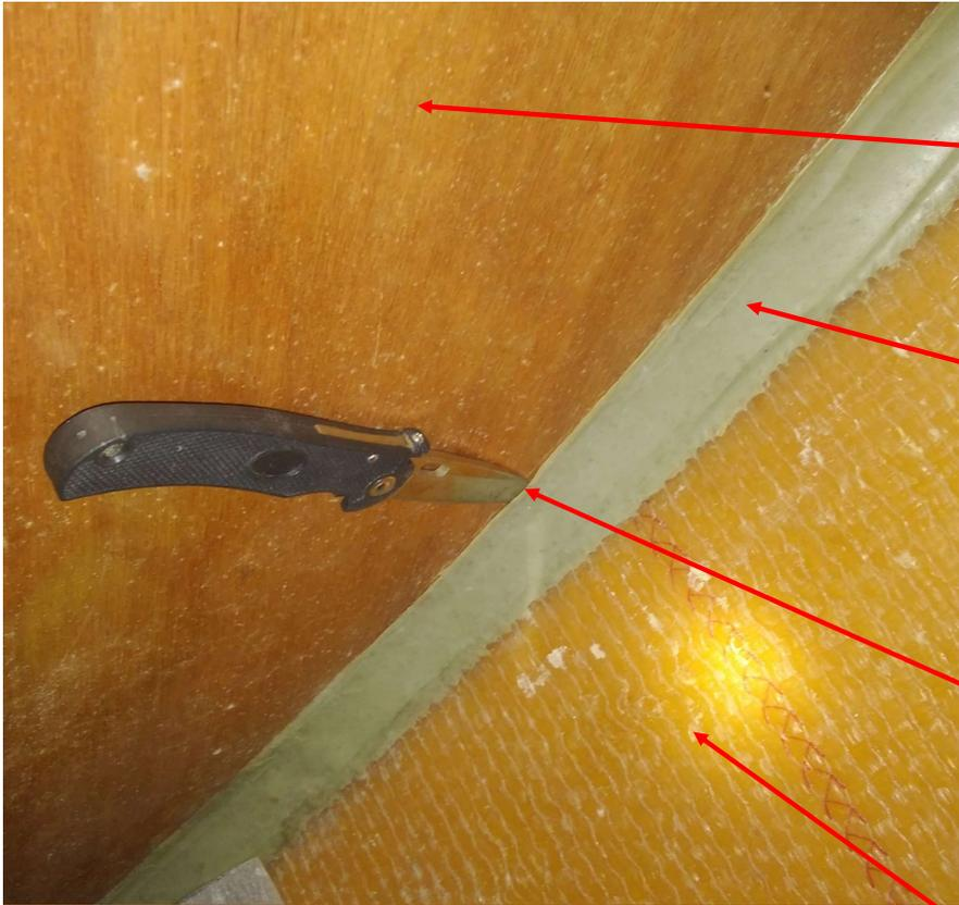
Solid plywood bulkhead with OEM varnish. Approximately 16 mm thick and roughly 838 mm tall. This one is under the berth in a forward cabin.
