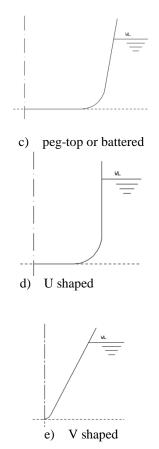
Figure 46: Typical shapes of transverse ship sections
