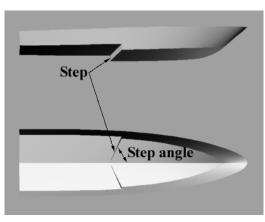
Figure 54: Step in planing craft hull
