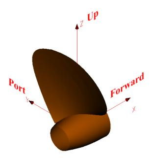
Figure 42: Propeller reference system, rectangular
