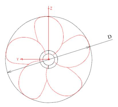
Figure 38: Propeller disk, looking forward
