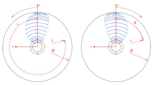
Figure 41: Propeller reference system, cylindrical, looking forward
