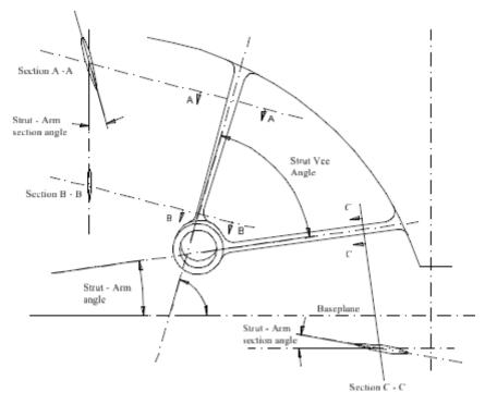
Figure 56: Characteristics of propeller strut or shaft bracket
