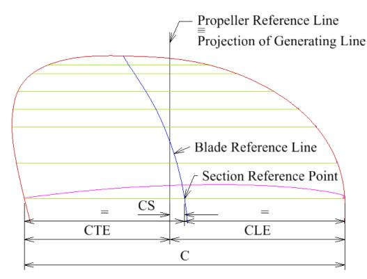
Figure 21: Portion of an expanded blade of a right handed propeller, showing Chord subdivision.
