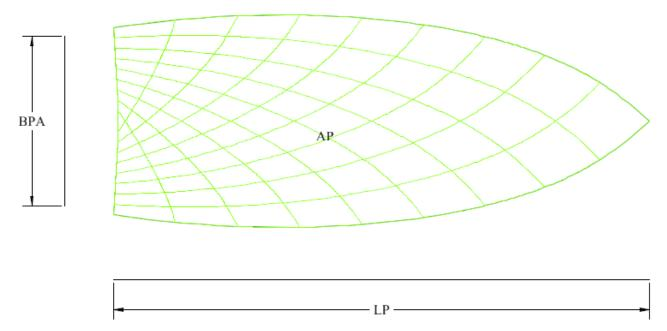
Figure 11: Mean beam over chines
