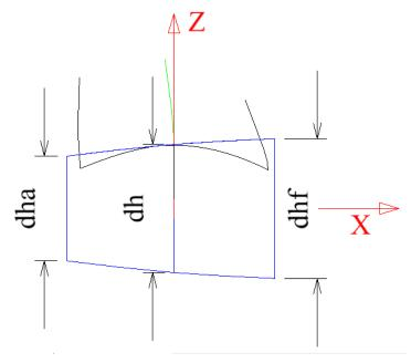
Figure 29: Hub diameters
