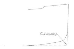
Figure 24: Cutaway at fore end of ship
