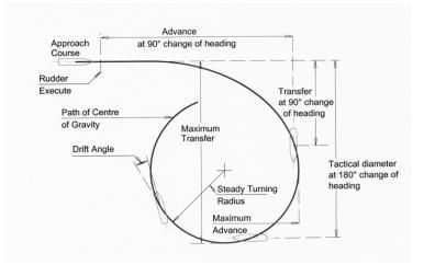
Figure 1: Geometry of turning circle
