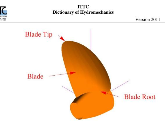
**Figure 12: Propeller Blade**
