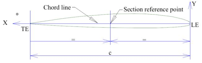
Figure 15: unrolled generic propeller blade section
