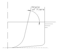
Figure 27: Transverse ship section with flare
