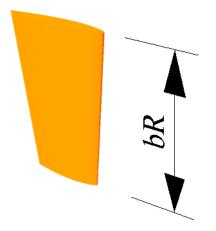
Figure 44: Rudder span
