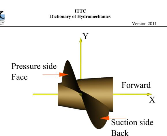
**Figure 36: Propeller blade surfaces**
