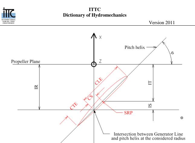
Figure 20: View of unrolled cylindrical section at radius r of a right-handed propeller (looking down) showing subdivisions of the Chord, Skewback and Rake.
