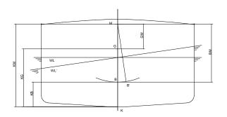
Figure 35: Transverse metacentric parameters
