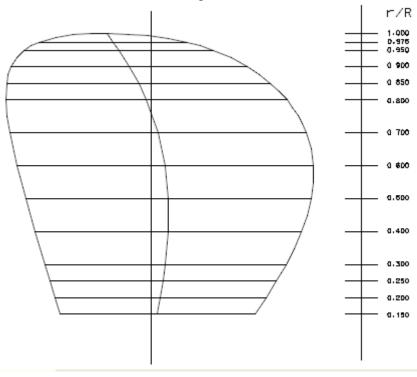
Figure 4: Expanded area of a propeller blade
