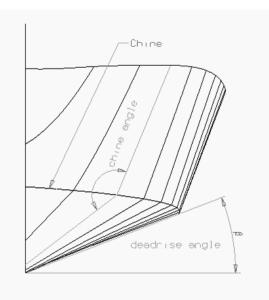
**Figure 19: Hull form with chine**
