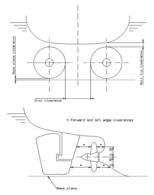
**Figure 22: Propeller clearances**
