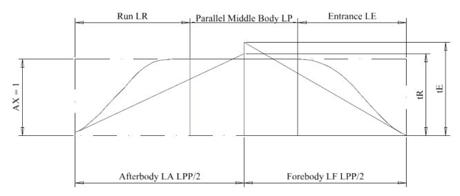
Figure 47: Characteristics of sectional area curve
