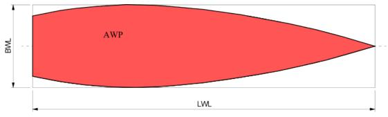
Figure 58: Waterplane area coefficient
