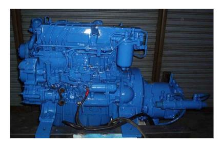
Base is a Isuzu 4JB1 M second hand marine diesel engine. The engine is coupled to a Koysan Hydraulic Marine Gearbox H4. This propulsion unit is going to be installed in a 25 foot inshore fishing boat in Malaysia and drives a Levi Drive LD 170-150.
