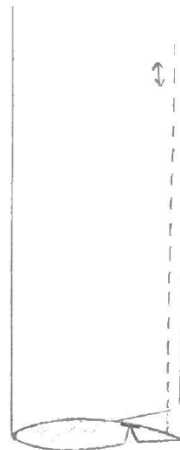
Figure 8.2 A flap with a fiberglass hinge.
