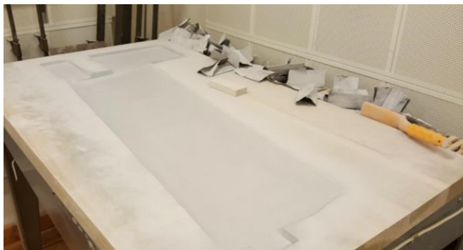
Figure E.3 The right centerboard strut mold-half.
