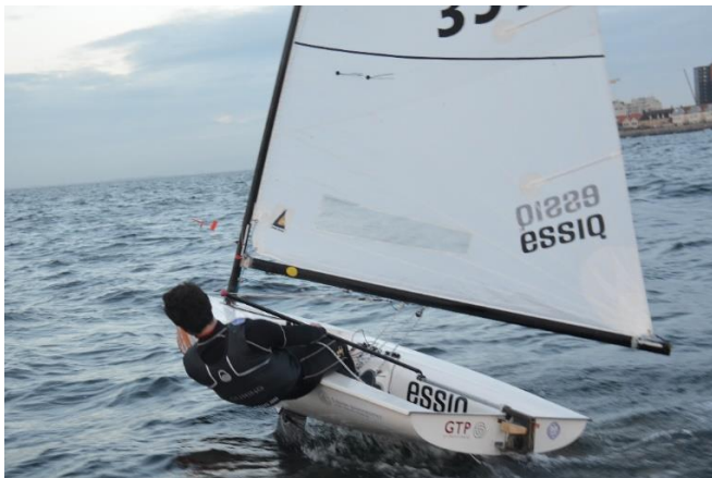
Figure 13.7 The centerboard foil creates enough lift to foil, but the rudder foil does not.
