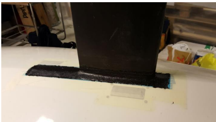
Figure E.21 Creating the plateau around the centerboard strut.
