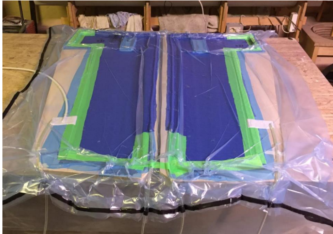
Figure E.8 The molds covered with the vacuum bag.
