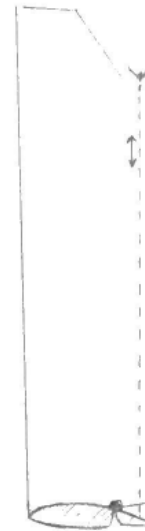
Figure 8.5 A flap with a mechanical hinge.
