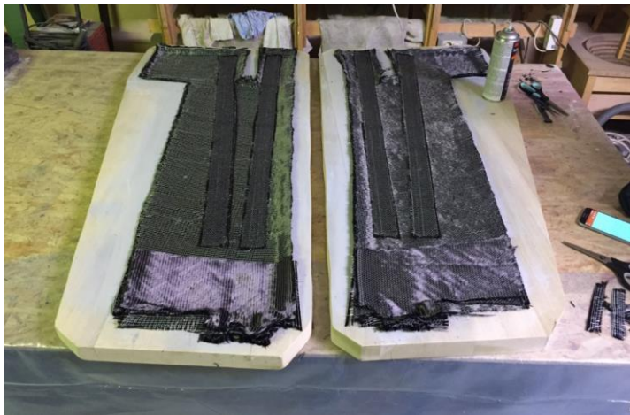
Figure E.4 Arrangement of carbon fiber.
