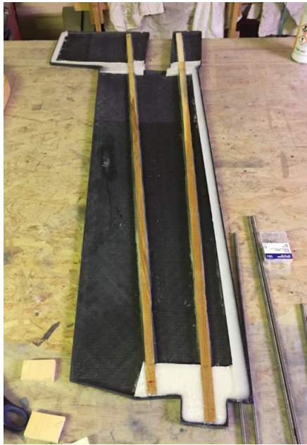
Figure E.18 The centerboard strut with a brink along the leading edge.
