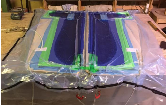
Figure E.9 Epoxy spreading among the fibers.
