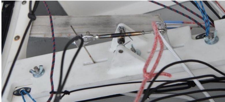
Figure E.22 The plate fitted to the centerboard case.
