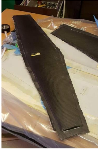
Figure E.15 The rudder foil with molding flashes.
