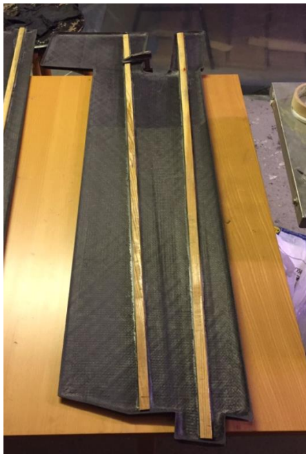
Figure E.17 The centerboard struts fitted with beams.
