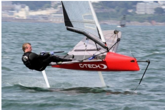
Figure 7.2 A moth with the wand fitted to a bowsprit [32].
