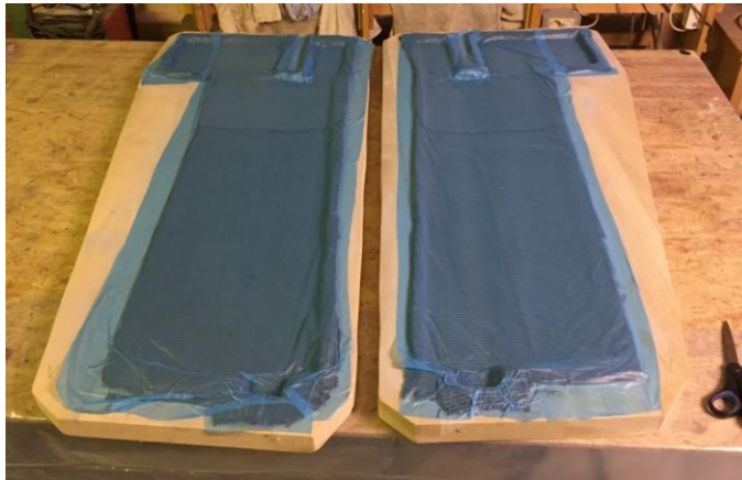
Figure E.6 The carbon fiber covered with the peel ply.
