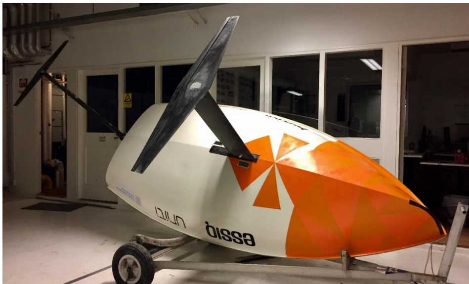
Figure 13.5 The centerboard and rudder fitted to the hull of the Europe-dinghy.
