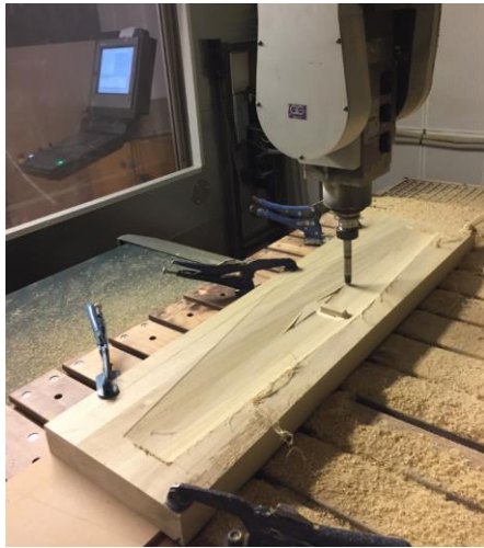
Figure E.2 CNC milling one of the molds.
