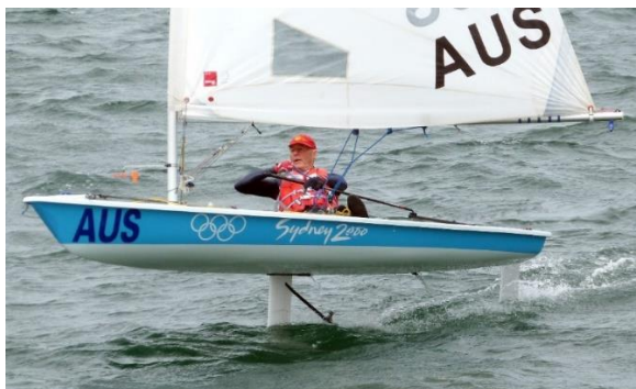
Figure 7.3 The foiling laser with the wand integrated in the centerboard [33].
