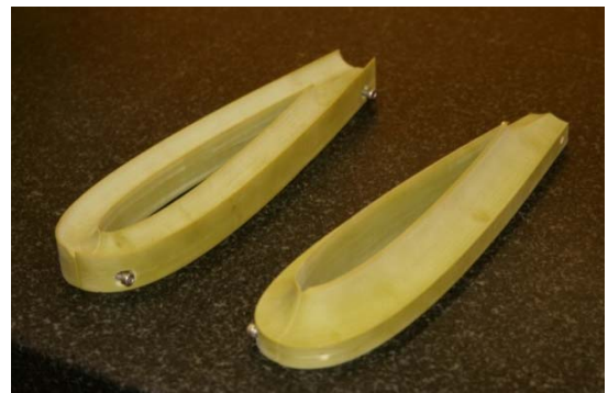
Figure 3 The top image is a schematic of the deflectors, the quarter circle is fitted to the strut. The bottom image shows the half circle, 180^\circ , (left) and quarter circle, 90^\circ , (right) deflector attachments.
