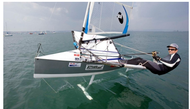
Figure 1 A Moth dinghy on hydrofoils. Photo courtesy of Thierry Martinez, © www.thmartinez.com.
