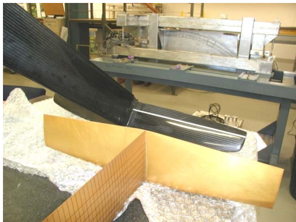
Figure 2 The tested T-Foil dimensions are shown in the top image. Actual foil is shown in the foreground of the lower image. Actual Moth rudder T-Foil is shown behind. Force balance can be seen in the background.
