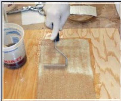
return a few minutes later, the laminate appears to be drying out, even though there's no sign of resin sag or drainout. This continues right up until the resin gels, and then I don't like the way the tabbing looks. What's going on?"
