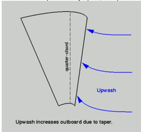
A tapered wing has a much shorter tip section than root section. As the wing tapers, lift produced by the shorter outboard sections is less because they have less surface area to support lift. Since the outboard sections are smaller than the inboard sections, they are significantly influenced by the larger wing just inboard. Air approaching the outboard portion of the wing is deflected by the low pressure on top of the
