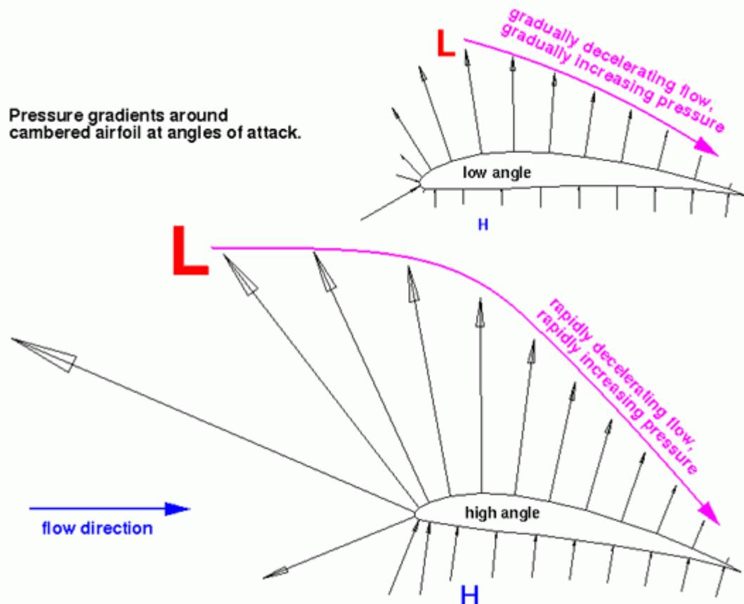
As the flow slows down from its accelerated state on the leeward side it yields a pressure gradient along the back of the sail that is increasing from very low pressure (to produce the desired lift) to a much higher pressure toward the leech. The amount of initial acceleration (dependent on angle of attack and shape) and the length of the pressure recovery determine how steep this gradient is. When the increase
