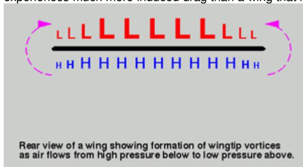
The most effective way to minimize induced drag is to increase span, as induced drag is inversely proportional to the span squared. Highly efficient airplanes like gliders have very high span for the amount of lift they are producing. Winglets are a way to create the effect of higher span without actually increasing the physical span. They are useful when there is an artificial constraint on wingspan (like a draft limitation on a keel).
