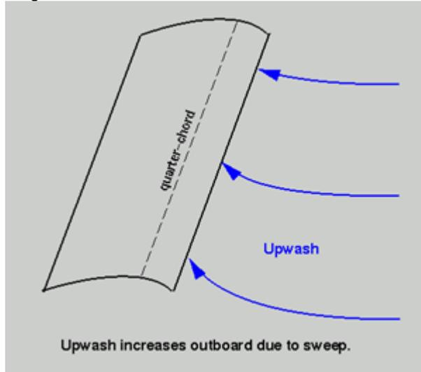
Sweep has the effect of increasing the upwash on the outboard wing sections. As a wing is angled aft, flow over the outboard sections must pass by the low pressure on top of the wing sections immediately inboard and forward. The close proximity of that low pressure to the air just outboard causes the outboard flow to turn upward more, resulting in higher upwash on the outboard wing.
