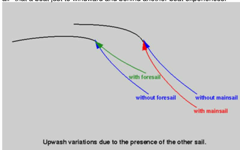
The mainsail of a sloop rig operates in the downwash of the forward sail, causing the flow angle
