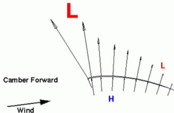
**Camber forward produces lower pressure forward and smoother deceleration over a longer distance.**
