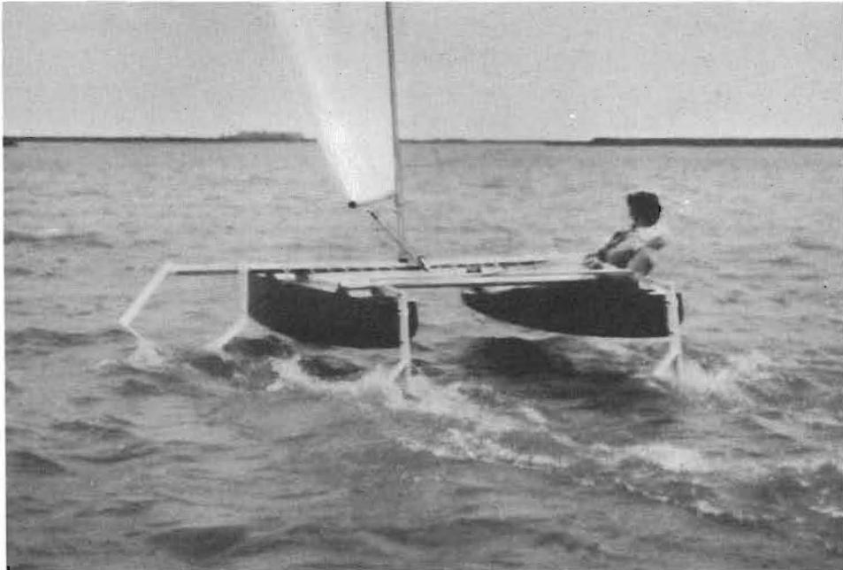
Fig. 51 Hansford's boat, showing twin rudder foils
