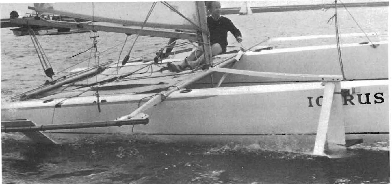
*Fig. 48 Close-up of Icarus, showing mechanism for 'tip-over' (photo Yachting World)*
