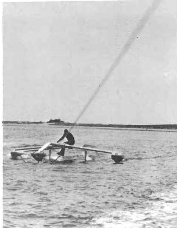
Fig. 36 Tow-testing Bradfield's 1967 version
