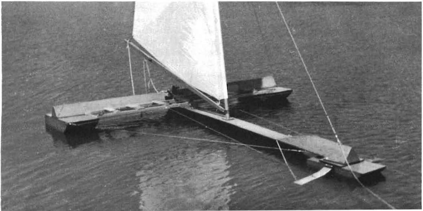
The original boat of figs. 30 and 31 was 17 feet long overall and had a 14-ft beam. It weighed 218 lb. all up, and had a  $6\frac{1}{2}$ -knot take-off speed requiring 13 knots of wind. Design calculations indicated a speed of about twice the true wind speed on its fastest point under favourable conditions. The hydrodynamic design was optimized for the 20 to 30-knot speed range.
