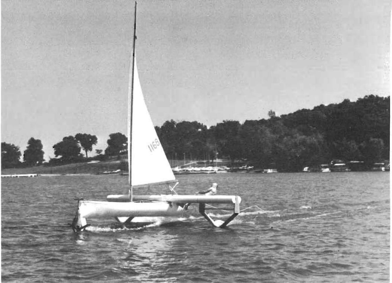
*Fig. 40 Flying Fish, showing front foil at high speed*
