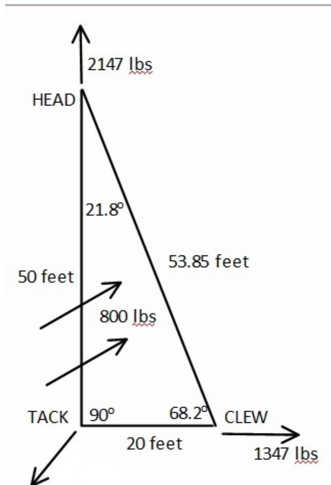
The force on the head is roughly the sum of the wind pressure on the sail pulling the sail down, and the load on the clew of the sail pulling back and down. In our example, with 800 pounds of wind pressure on the sail and 1347 pounds of clew load, we arrive at around 2147 lbs of load on the head.
