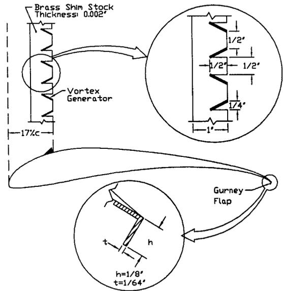
Fig. 15 Vortex generators and Gurney flap geometries used separately on the S1223 airfoil.
