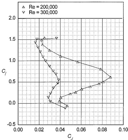
Fig. 9 Drag polar for the M06-13-128 airfoil.
