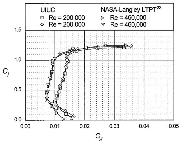
Fig. 4 Comparison of the E387 measured drag polars.
