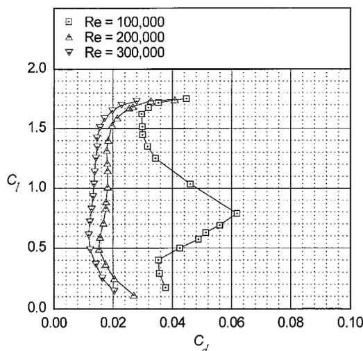
Fig. 6 Drag polar for the FX 63-137 airfoil.
