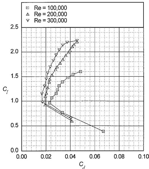
Fig. 18 Drag polar for the S1223 airfoil.
