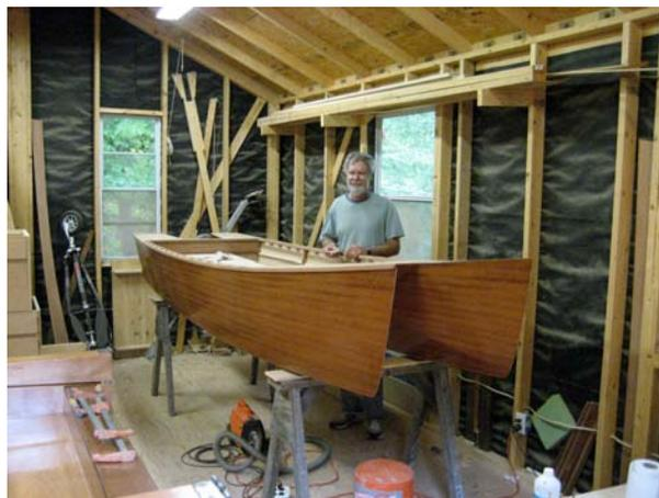
dory construction, using 1/8" plywood sides and decks, stringers, and 1/4" plywood bottom and seat. I veneered the hulls sides and decks with ribbon grain mahogany just for fun. If you would like more information on how to do this, please contact me. Here are the basics of building Glider.
