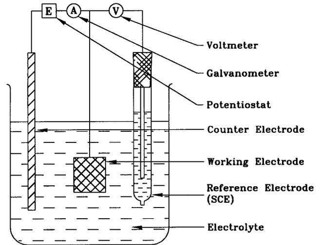
FIG. 4. Schematic of Electrical Circuitry for Polarization Measurement
