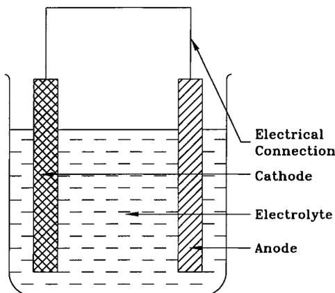
FIG. 1. Schematic of Basic Wet Corrosion Cell
