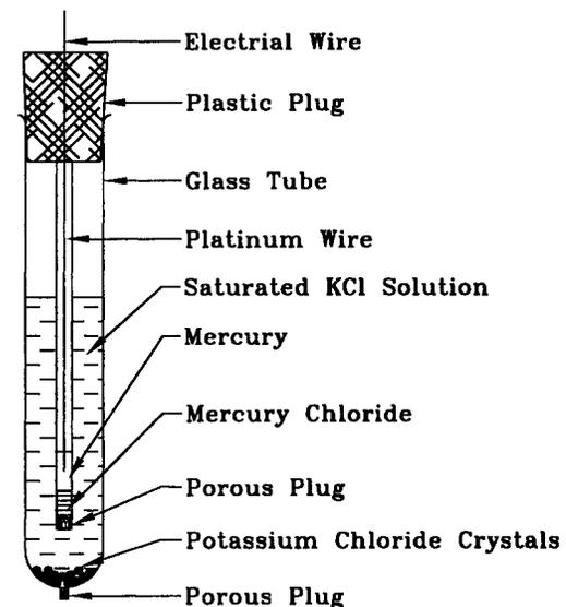
FIG. 2. Schematic of Saturated Calomel Electrode (SCE)
