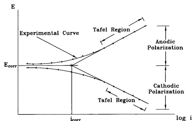
FIG. 3. Typical Polarization Result Showing Tafel Extrapolation
