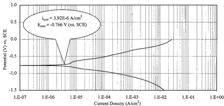
**FIG. 10.** Polarization Curve for Steel in Seawater
