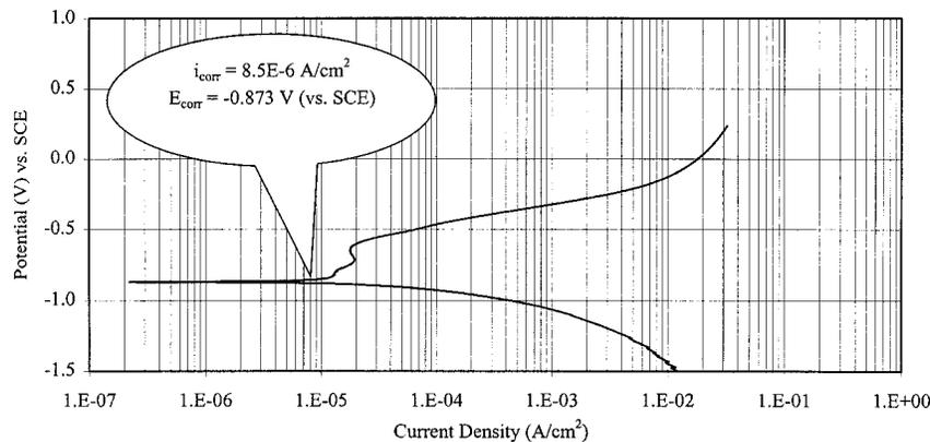
**FIG. 9.** Polarization Curve for Steel in Deicing Solution
