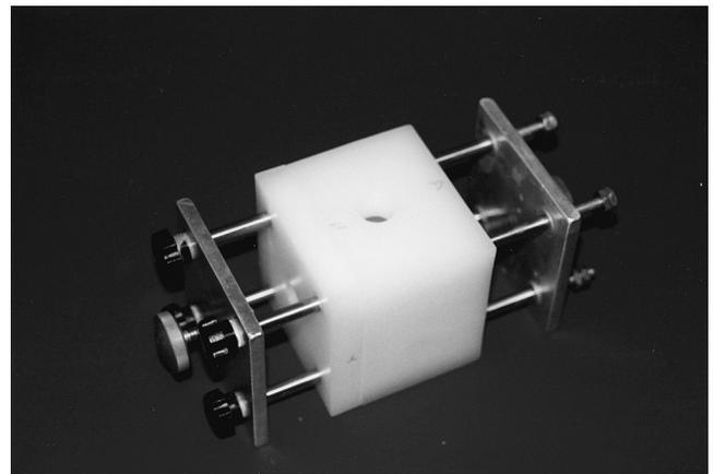
FIG. 8. Flat Cell Used in Corrosion Testing
