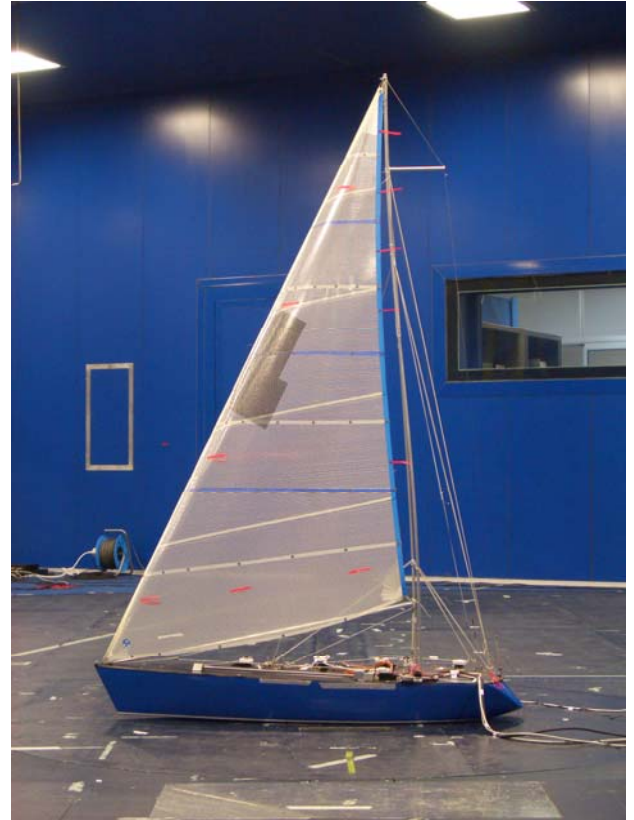
Figure 12. Single jib configuration during the test
