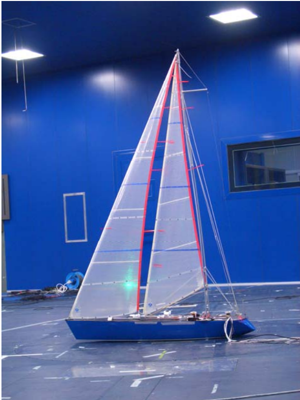
Figure 11. Double jib without overlap configuration during the test
