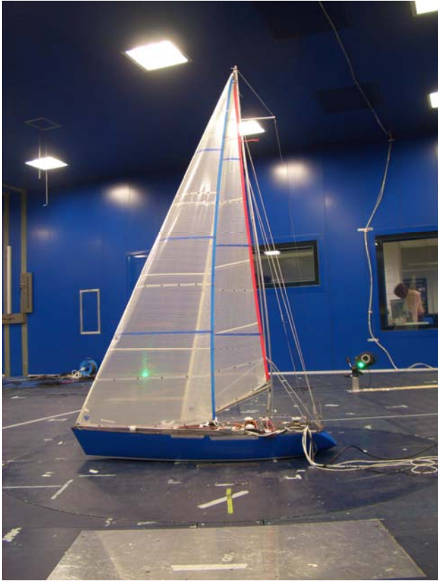
Figure 10. Double jib with overlap configuration during the test
