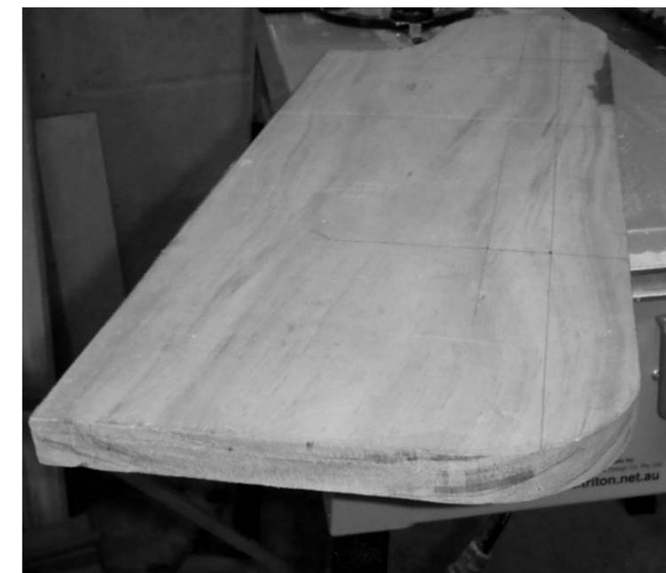
You will observe it has been cut from a single plank of back sawn timber which has naturally warped already (The annual rings of the timber tend to
