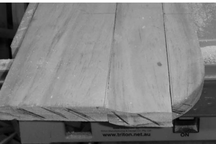
The joins are dowelled together and epoxy glued the cramped together for 24 hours. To keep the board flat, I clamped it to a piece of shuttering plywood covered with packing tape to prevent adhesion to this base.
