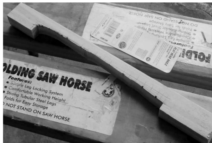
The finished test piece is then used to confirm the section of the foil as it is shaped with plane, spokeshave and sander. To ensure that the foil lasts, we will be sheathing it in fibreglass, so it is acceptable for the timber to be up to 1mm undersize to accommodate resin and mat.
