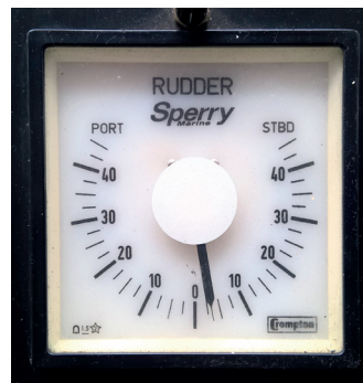
Figures 5/6: The "Rotor Control" display (left) shows a rotor side force of 39.1 kN (circled in red) acting on the ship. The rudder angle indicator (right) shows that a rudder position of only about 3^\circ to starboard is required to keep the ship on course with autopilot control. Source: Hochschule Emden/Leer, University of Applied Sciences
