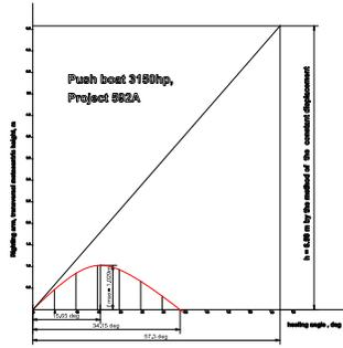
Ship with 10% store and fuel, 100% ballast in forepeak and damage afterpeak
