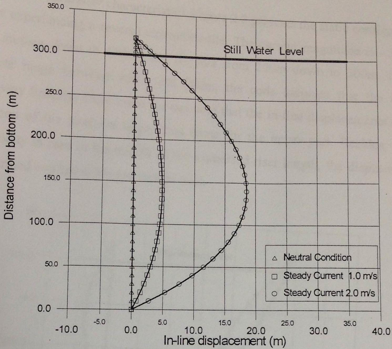
Figure 2.6 - Geometric Configurations for a Vertical Riser under Uniform Current
