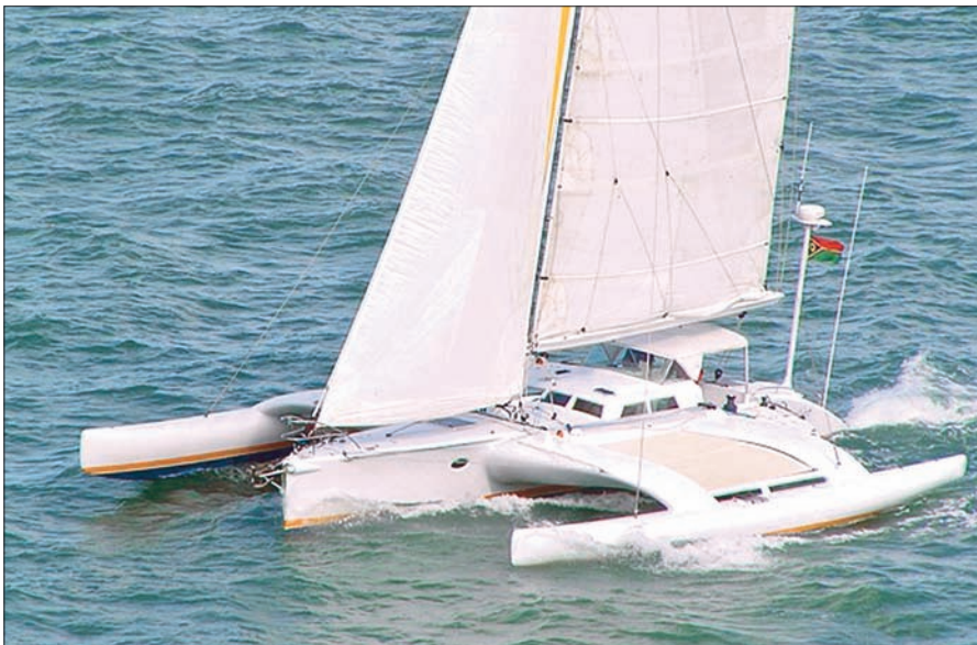
The 51' (15.5m) Traveller is a Corecell/E-glass/epoxy wing-mast sloop built in Brisbane, Australia, in 2003, and currently based in Auckland, New Zealand. The owner, an experienced transatlantic sailor, cruises Polynesia shorthanded; 300+ mile days are common. A sister-ship won the doublehanded Round Britain & Ireland Race, in 2006.
