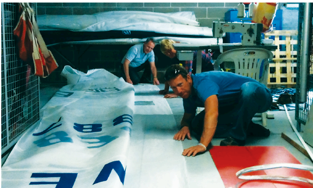
Re-cutting the luff curve of a mainsail in Freddy's basement at lake Garda. Freddy eyeballing the curve, in the background sailmaker Pelle Kindberg and Max Salminen's blond hair. Pelle is in charge of the production of all the One Design sails at WB.
