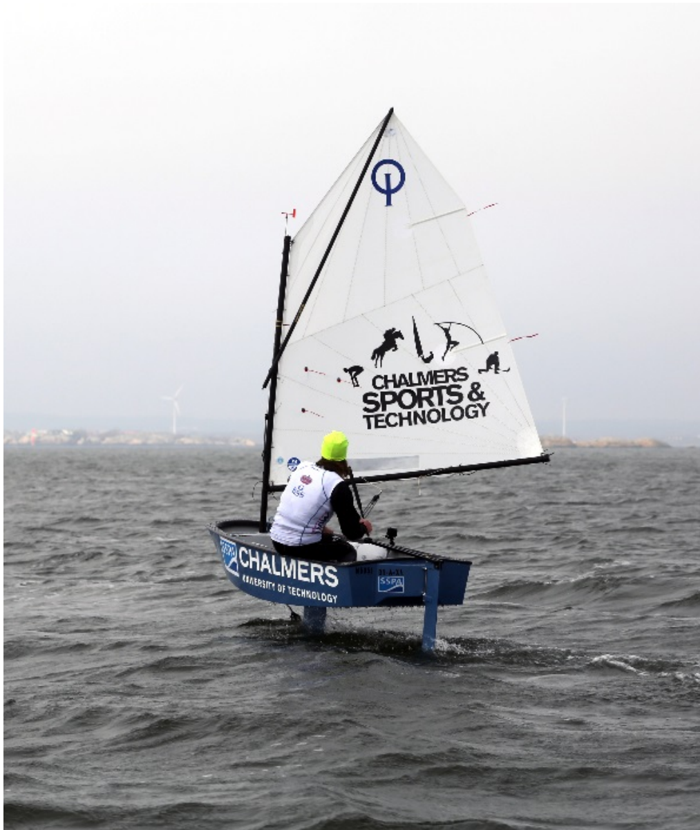
Figure 14. The foiling Optimist. Photo: Per Thorén
