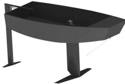
Figure 1. Optimist with foils and wand.
