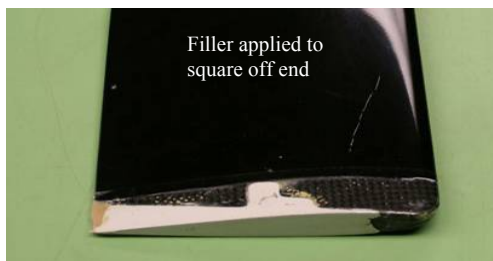
Figure 14 – Prismatic Strut Ends
