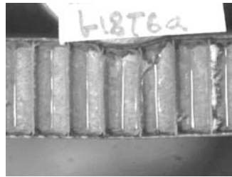
(c) Core crushing ( \rho_c = 128 \text{ kg/m}^3 , L = 60 \text{ mm} )
