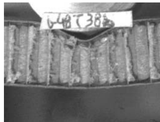
(b) Face wrinkling ( \rho_c = 48 \text{ kg/m}^3 , L = 380 \text{ mm} )
