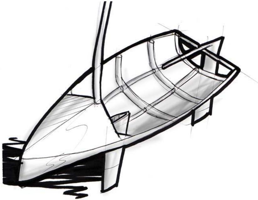
The hull comprises of a flexible plastic skin with inflatable ribs and forward buoyancy tank to give maximum strength and rigidity while allowing for easy disassembly.
