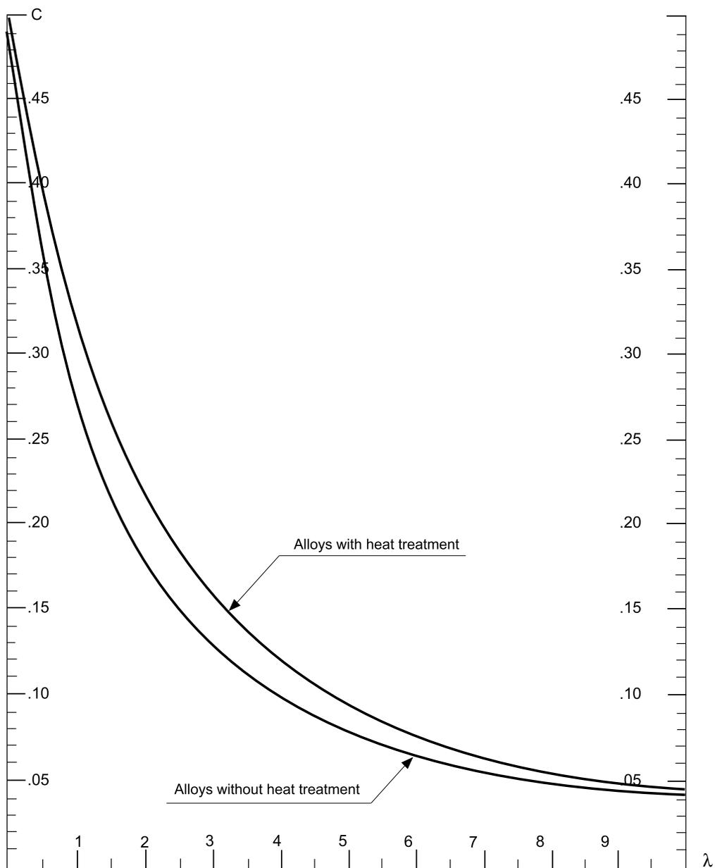
Table 4 : Buckling check of aluminium pillars subject to compression axial load
