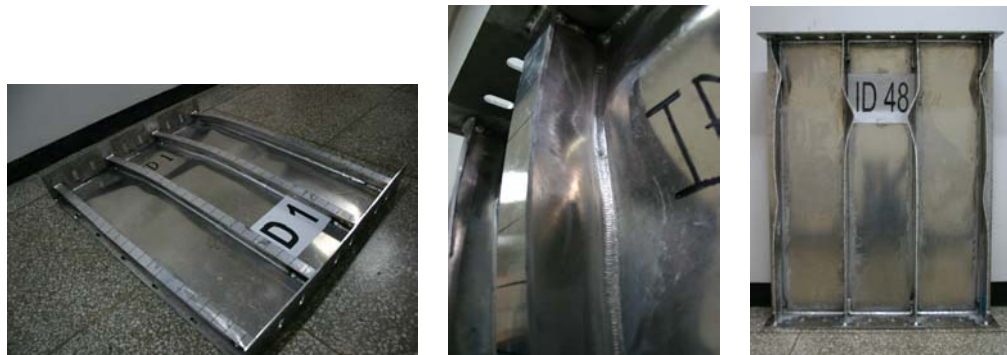
Fig 13 Typical collapse modes observed during the buckling collapse testing on aluminum plated structures
