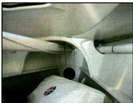
Detail view up forward in a Rip Tide 35, showing the deck and topsides arch support, and retractable bowsprit. A self-draining locker forward of the bulkhead contains any leaks around the sprit.
