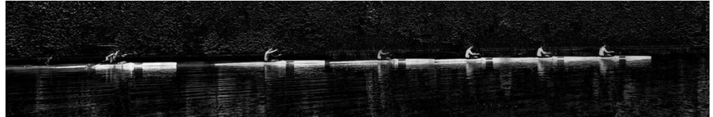
Figure 5. Chronophotography illustrating a deceleration test performed with L to measure the effective mass M_e via the deceleration of the boat. The time between each frame was \Delta t = 0.167 s.
